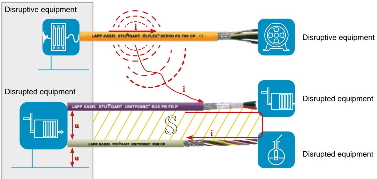
**In radiation, interference coupling can be created by an inductive effect.**
