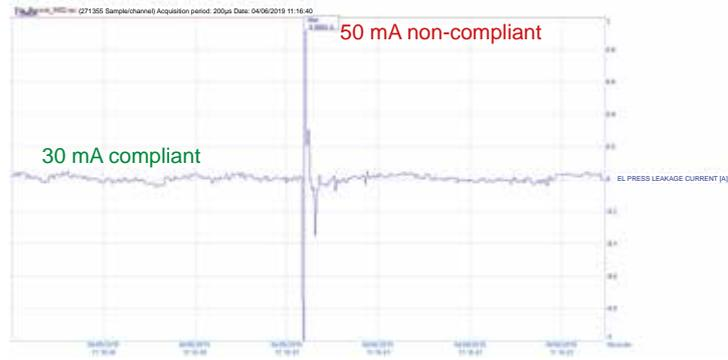
The modernisation of electrical installations leads to an increase in leakage currents. These leakage currents are created by parasitic capacitance caused by power electronics (e.g. variable frequency drives).
