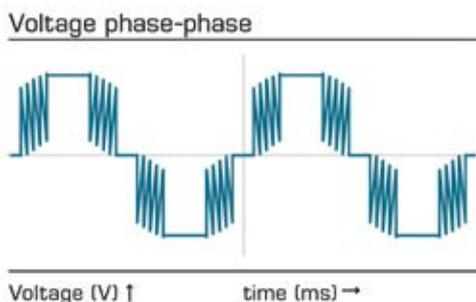
drive output signal phase-phase voltage with motor reactor
