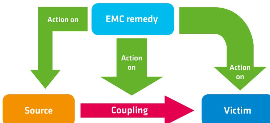
The evolution of technologies has made equipment more sensitive and therefore vulnerable to EMI damage. The wiring rules must be taken into account to avoid errors and therefore the risk of interference. In EMC, there are 2 propagation paths (coupling).
