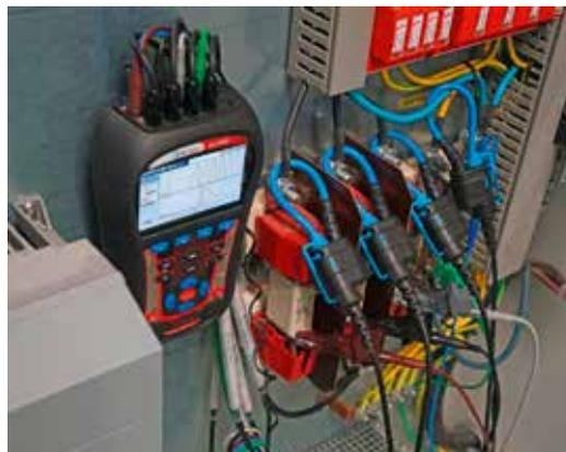
\* VFD (Variable Frequency Drive): function designed to perform measurements on variable frequency drives where the motor speed is controlled by the change of frequency.
