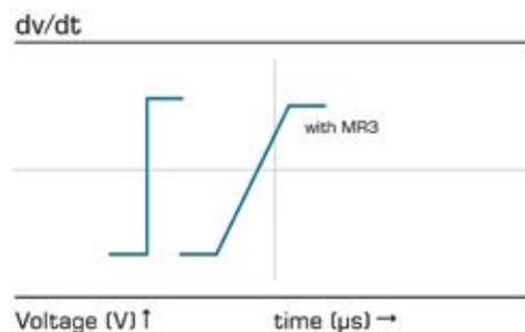
**Filtration with motor reactor to reduce dV/dt in differential mode**
