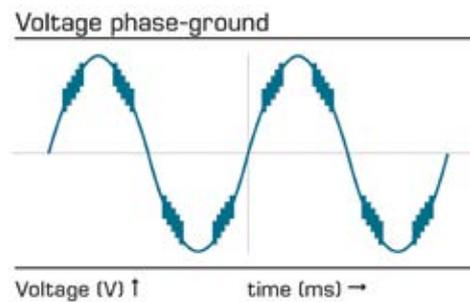
drive output signal phase-earth voltage with SF4 filter
