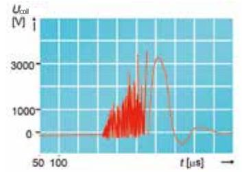
Overvoltage due to the operation of an auxiliary contactor coil not fitted with a 230 V, 50 Hz, 10 VA protection device
