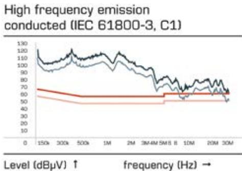
Unfiltered drive input HF signal
