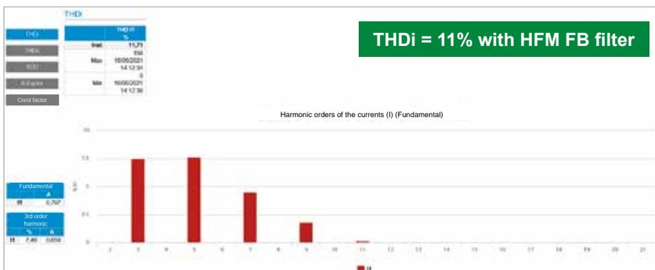
The result depends on several criteria concerning the installation. An analysis of the electrical network should preferably be conducted before and after filtration.
