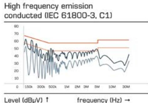
Filtered drive input HF signal
