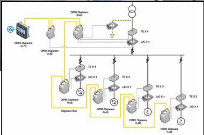
In accordance with standard NF C 15-100 relative to low-voltage electrical installations, constant monitoring by an RCM solution, such as the DIRIS Digiware RCM solution, means periodical measurement of the insulation resistance is no longer necessary.
