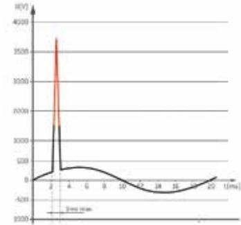
When the peak voltage reaches a value greater than the equipment can withstand, it causes its destruction
